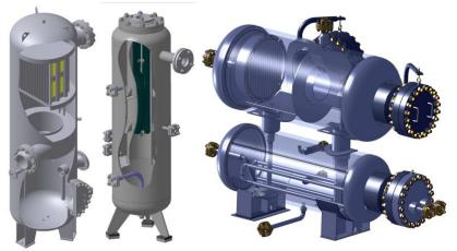
Gas separators of the inertial-filtering type are a unique type of equipment combining inertial and filtering methods of gas condensate systems separation. Combined separators are highly efficient gas cleaning from fluid in a wide range of productivity and pressure, provide long resource between regeneration and multiple regeneration, have low hydraulic resistance compared to the coalescing filters and even some gravity-inertial separators leading world manufacturers.
